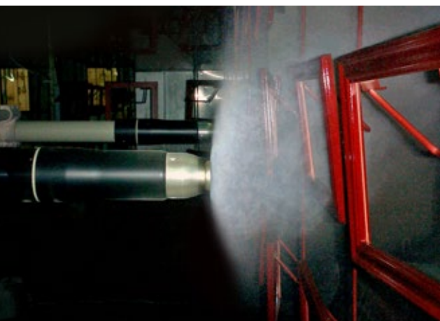
High speed bell, RPM 5,000 to 45,000 RPM, loaded
