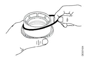
Insert the pressure rings with their seals into the valve body.
